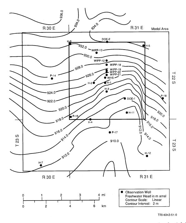
Figure 3-11. Best Estimate of the Undisturbed Freshwater Heads in the Culebra Dolomite Member (From Haug et al., 1987).
