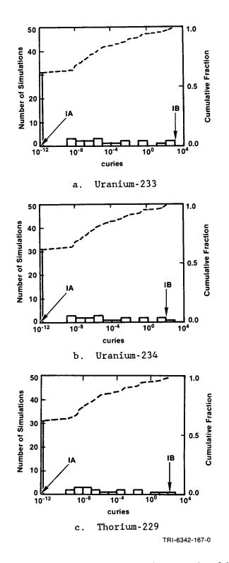
Figure 4-2. Histograms of Frequency of Simulations in which Quantities of Radioisotopes Migrate to the Base of the Shaft in 50,000 yr, Showing the Cumulative Fractional Density of Simulations, for Undisturbed Performance.
