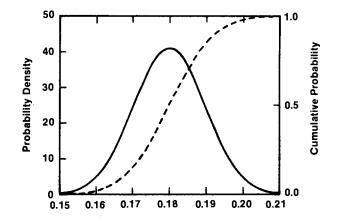
(c) Porosity: Normal Distribution Function for Cases El<sub>a</sub>, El<sub>b</sub>, El<sub>c</sub>, and El<sub>f</sub>, and Reference Design.
