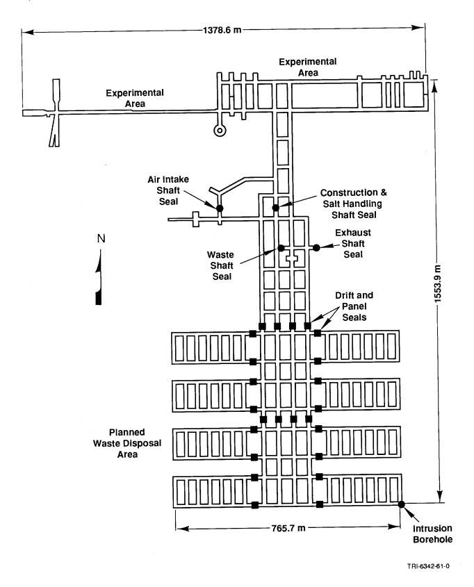
Figure 2-2. Location of Drift, Panel, and Shaft Seals (Modified from Lappin et al., 1989)
