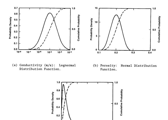
(c) Retardation: Beta Distribution Function (p = 1.762, q = 19.67) for Plutonium, Thorium, and Americium.
