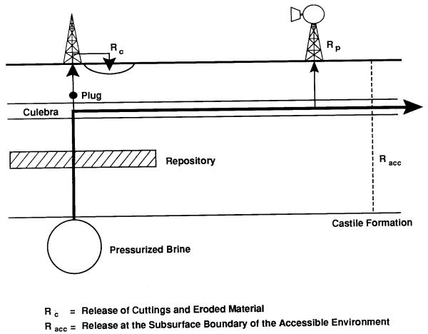
R<sub>p</sub> = Release to Surface through Withdrawal Well
