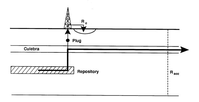
R<sub>c</sub> = Release of Cuttings and Eroded Material R<sub>acc</sub> = Release at the Subsurface Boundary of the Accessible Environment
