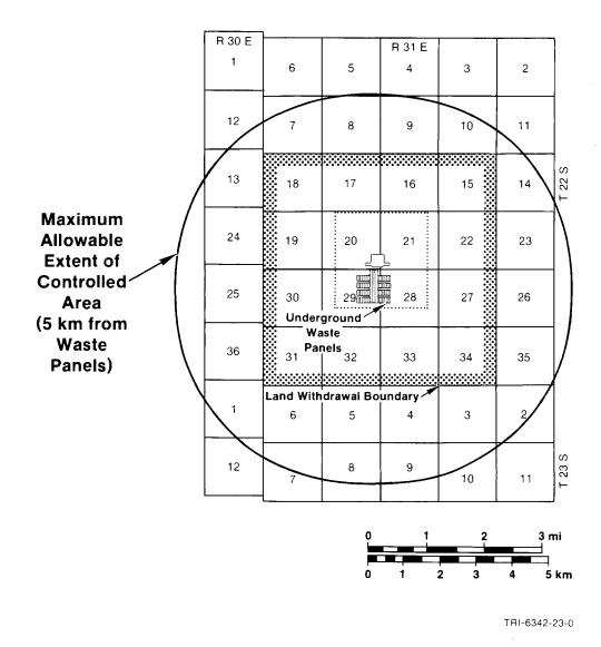
Figure 2-4. Location of the Underground Waste Panels Relative to the Proposed Land Withdrawal Boundary and the Maximum Allowable Extent of the Controlled Area Defined in the Standard (U.S. DOE, 1989b).
