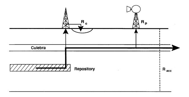
R<sub>c</sub> = Release of Cuttings and Eroded Material
