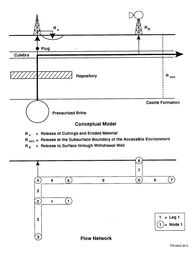
Figure 3-21. Conceptual Model and Flow Network for Scenario ElE3. Arrows Indicate Assumed Direction of Flow.
