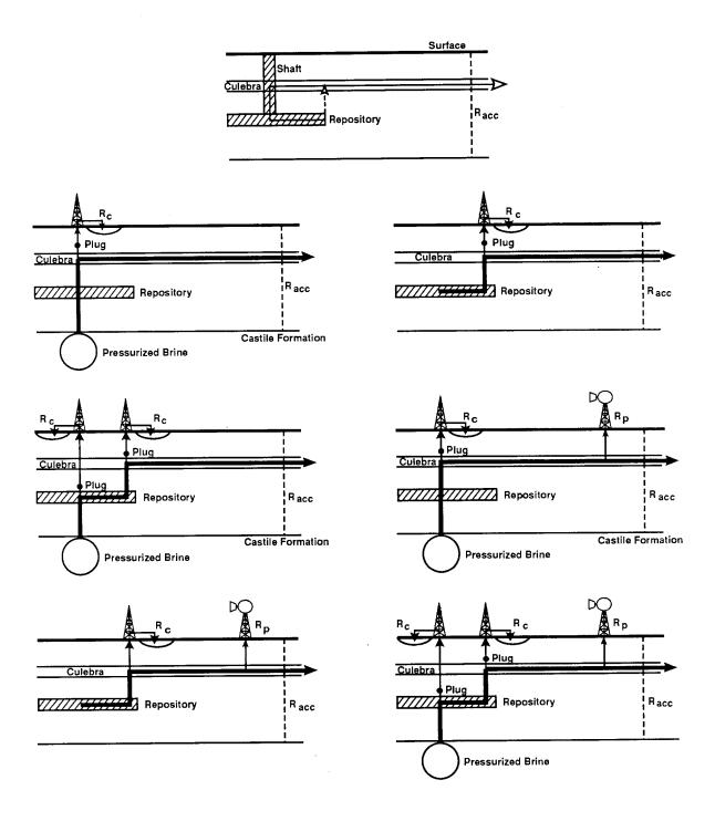
R<sub>c</sub> = Release of Cuttings and Eroded Material R<sub>acc</sub> = Release at the Subsurface Boundary of the Accessible Environment R<sub>p</sub> = Release to Surface through Withdrawal Well
