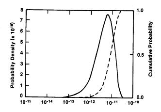
(b) Conductivity: Beta Distribution Function (p = 2.3953, q = 21.580) for Cases El<sub>d</sub> and El<sub>e</sub>, and Modified Design.
