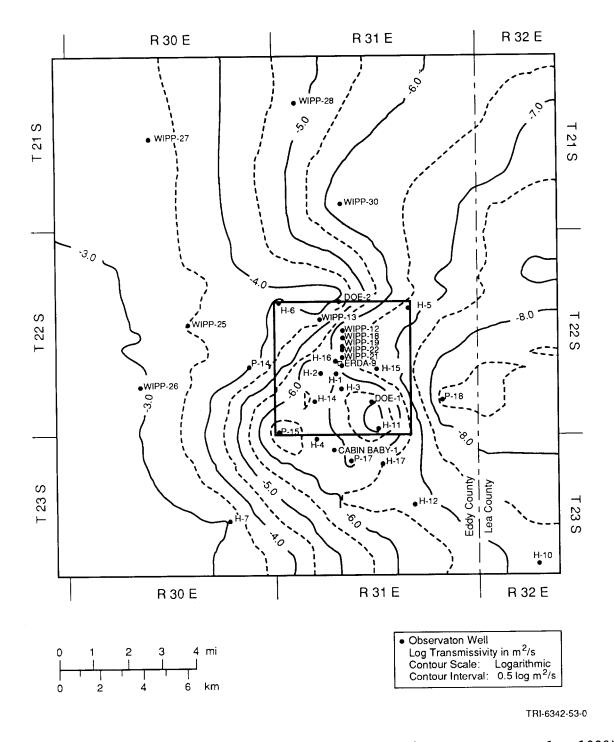
Figure 3-13. Kriged Transmissivities (Reproduced from LaVenue et al., 1988)
